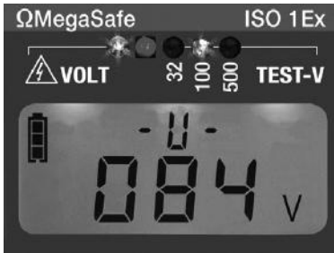
Charge voltage indication with external connected capacitance
