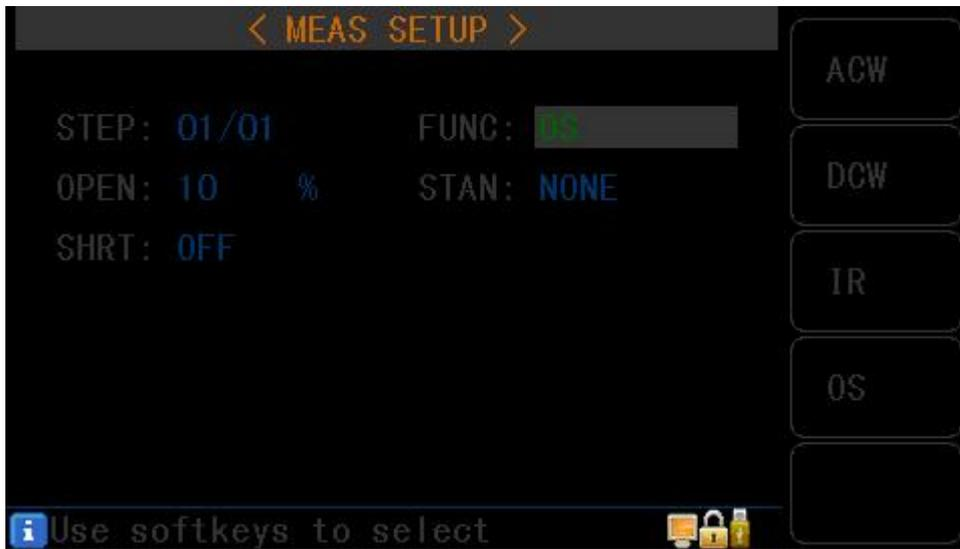
Figure 4.3.4 OS setup interface
