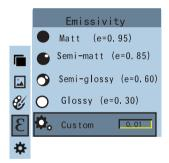
As shown in the figure, press "  $\oplus$ / MENU" key to enter the main menu and select "  $\pounds$  "(emissivity) option and press "  $\blacktriangleright$  " key to enter the emissivity list.
