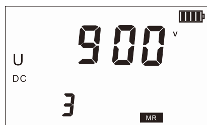
Figure 13-4 DC voltage check
