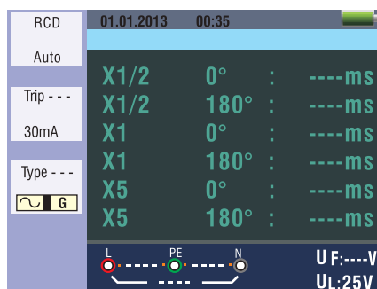
Figure 16 RCD Auto Function Screen
