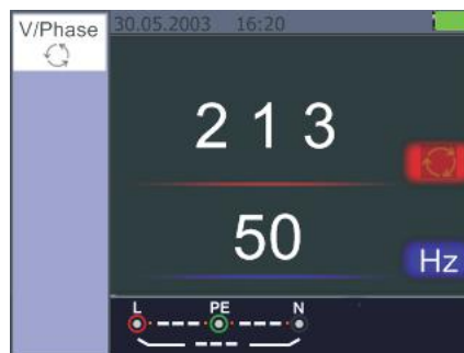
Figure 24 Phase Sequence-When connected in counter-clockwise manner
