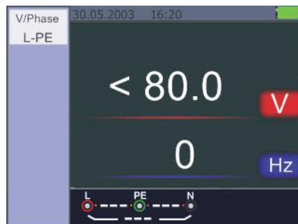
Figure 19 Standby screen for the Voltage and Frequency
