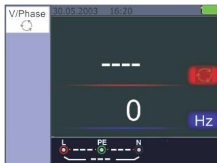
Figure 21 Initial screen of the Phase Sequence Measurement
