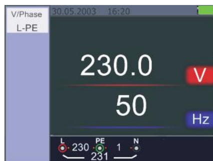
Figure 20 Screen while measuring Voltage and Frequency
