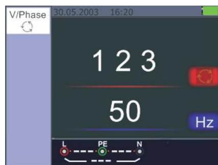
Figure 23 Phase Sequence screen-when connected in clockwise direction.
